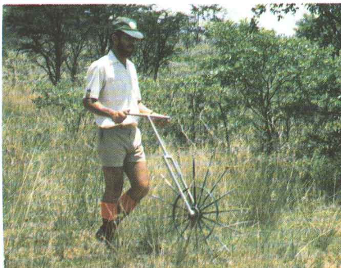
A wheel-point apparatus used to randomly select sample points (Tidmarch & Havenga, 1955).
