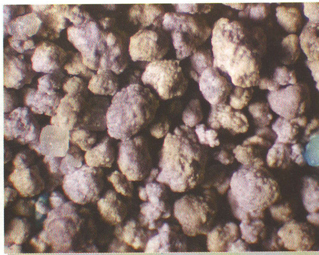
Mixture of 1:5:94 salt, CuSO 4 and P18 (stereo)
