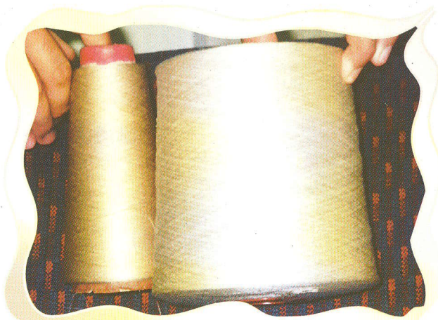
Silk yarn. Left - pure silk, right a blended yarn - 20% silk, 80% wool. Note the colour and shine.
