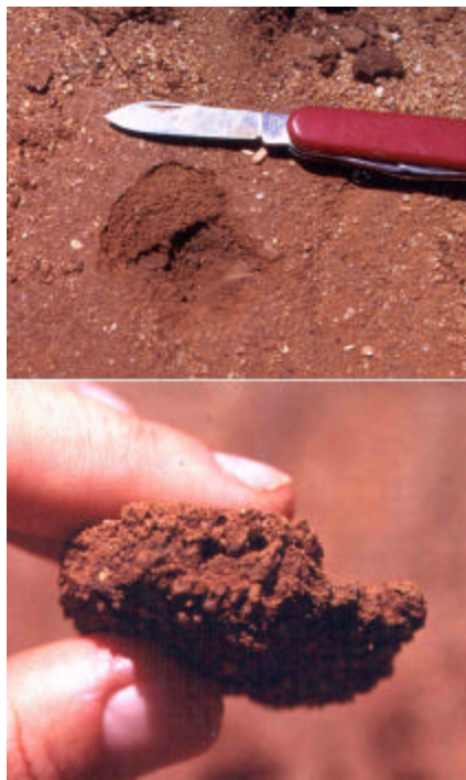
Figure 12: Air bubbles are cemented into the crust of soils just below the soil surface by a thin clay layer. These air bubbles prevent the infiltration of water into the soils and thus create an arid soil climate. (Photo: B. Strohbach, Okahandja district, 1999)
