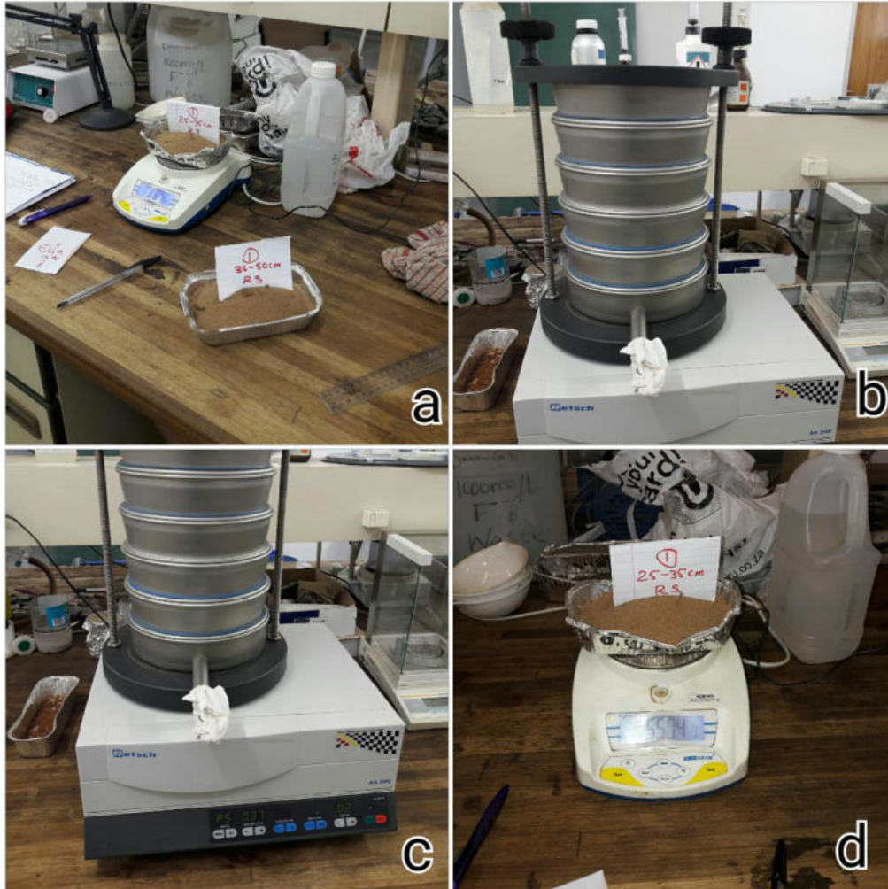
Figure 7. Sieve analysis at the University of Namibia’s Geology Laboratory: (a) Weighing unsieved samples from different depths; (b) and (c) Sieves stacked according to diminishing aperture; (d) Weighing each size fraction for classification of the soil
