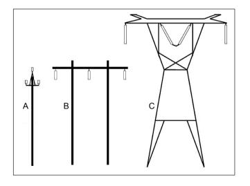
**Figure 2:** Typical configuration of (a) 11/22 kV distribution power lines, and (b) 66 kV and (c) 132/400 kV transmission power lines in the Overberg (not to scale), showing placement of conductors. Transmission lines also have overhead earth wires
