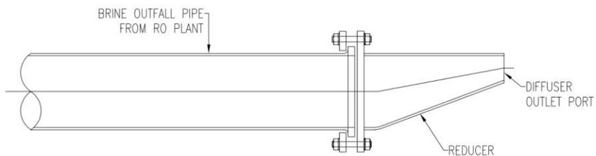
DIFFUSER SECTION: SURFZONE DIFFUSER
