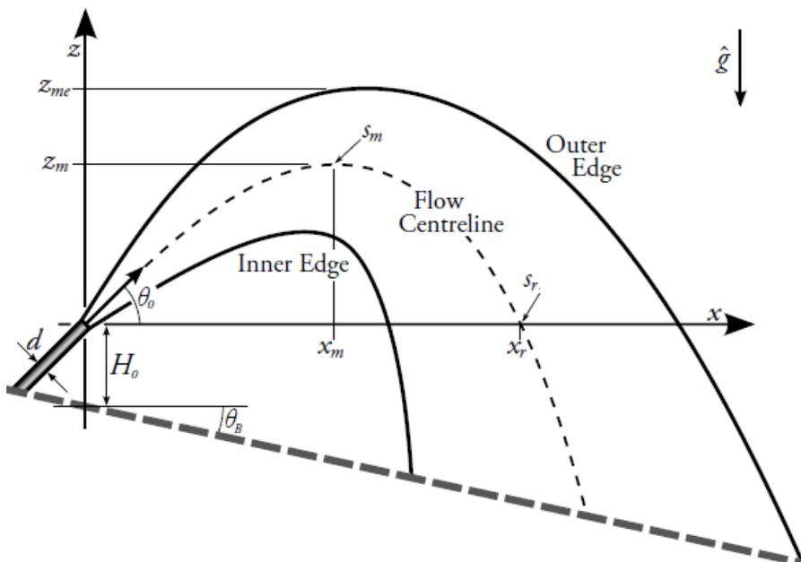
**Figure 3.1: Configuration and notation for an inclined negatively-buoyant jet (Oliver, 2012)**
