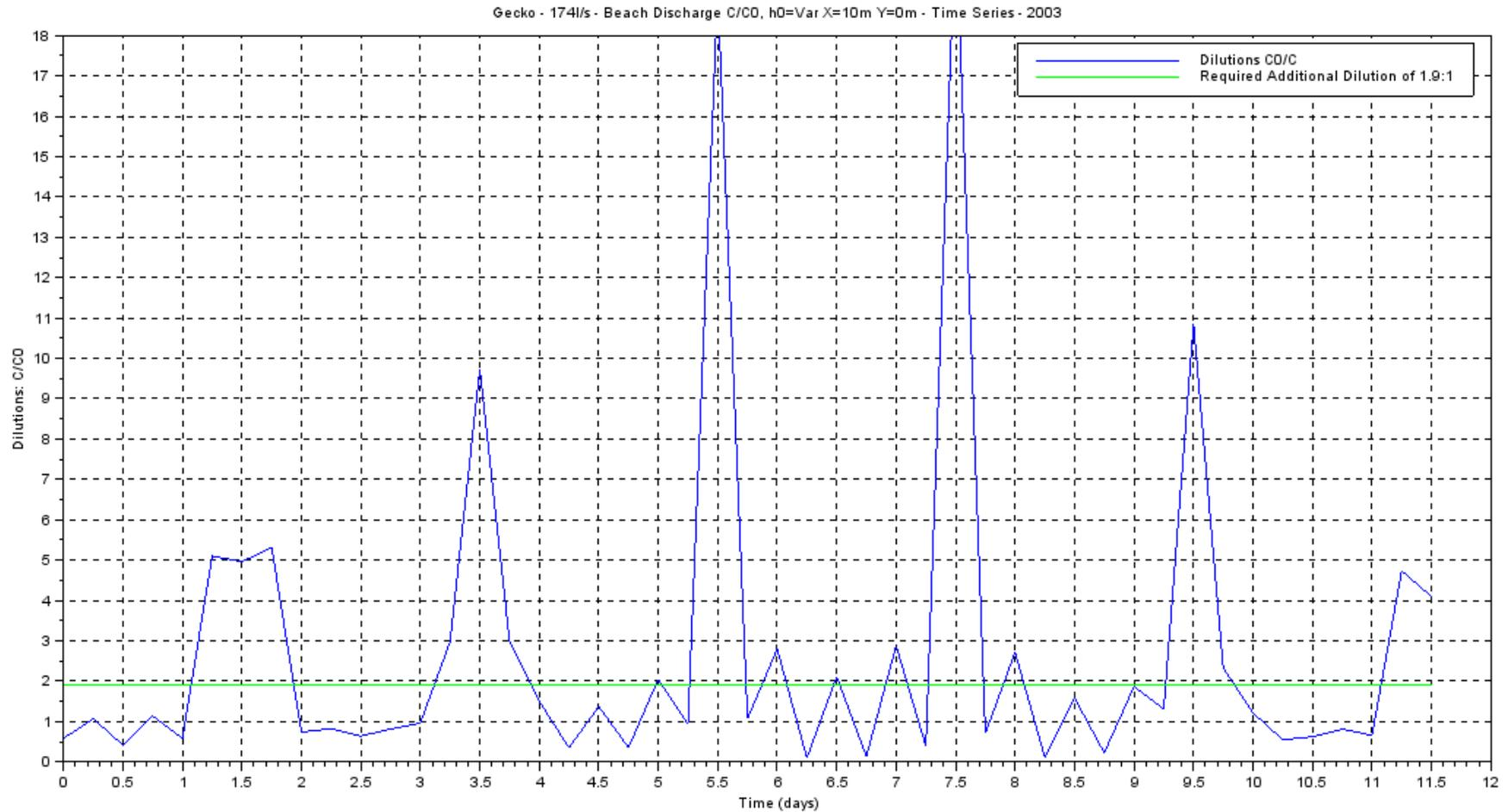
Figure 8.2: Plot of dilutions achieved for the 2003 time series calculated at a fixed point “B” (10m from the point of initial dilution) for the brine effluent discharge. The green line indicates the required dilution of  $D=1.9:1$ . The blue peaks below the line indicate dilutions below the required  $D=1.9:1$ .
