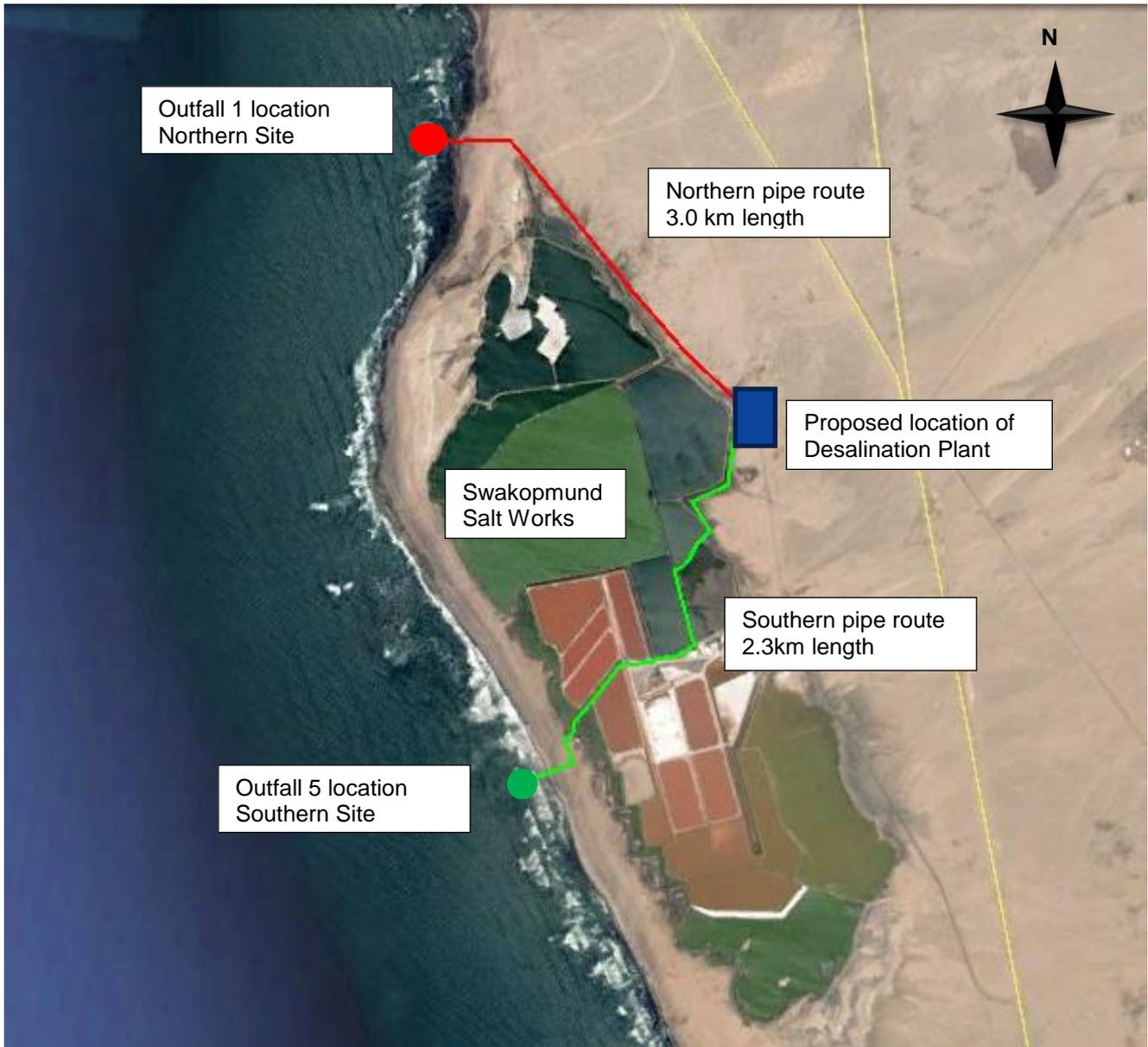
Figure 2.1: Layout of site and location of proposed and two outfall sites considered
