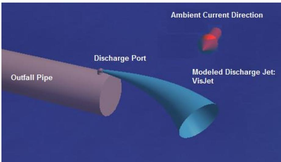
**Figure 5.1: VisJet model rendering of an outfall jet. The blue cone simulates the evolution of the discharge jet over distance. The red arrow indicates the current direction. Note that the pipe size rendering is exaggerated.**
