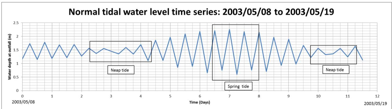
**Figure 6.1: Normal tidal water level time series: 2003/05/08 to 2003/05/19 representing the average wave conditions occurring at the site.**
