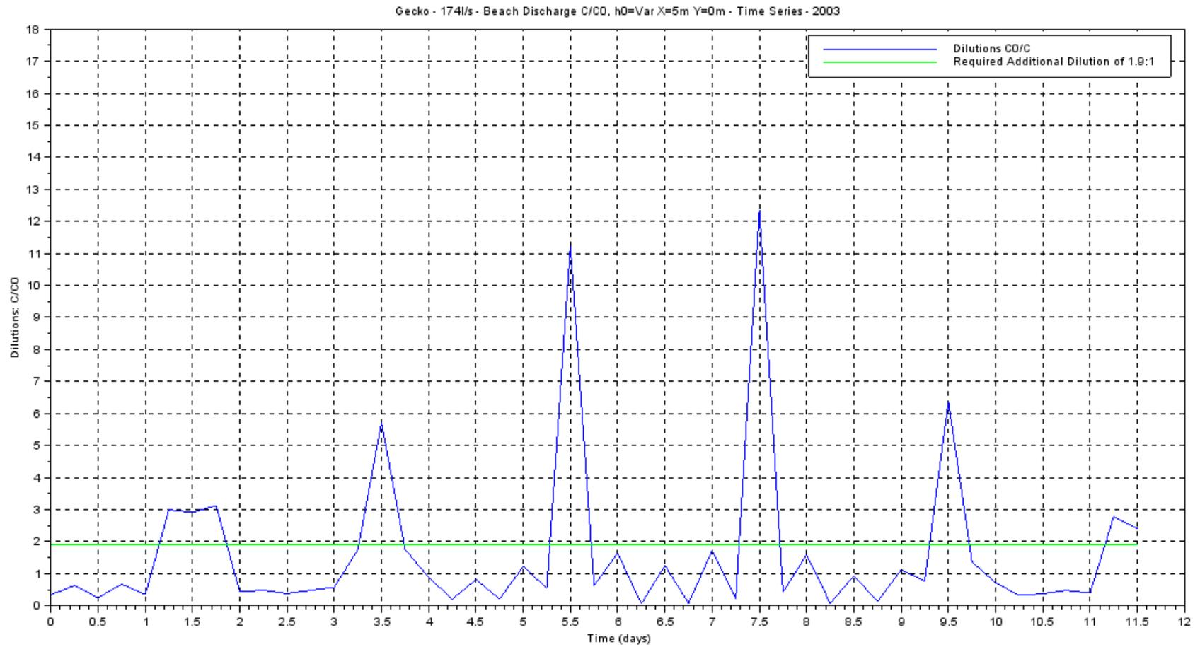
**Figure 8.1: Plot of dilutions achieved for the 2003 time series calculated at a fixed point “A” (5m from the point of initial dilution) for the brine effluent discharge. The green line indicates the required dilution of  $D=1.9:1$ . The blue peaks below the line indicate dilutions below the required  $D=1.9:1$ .**
