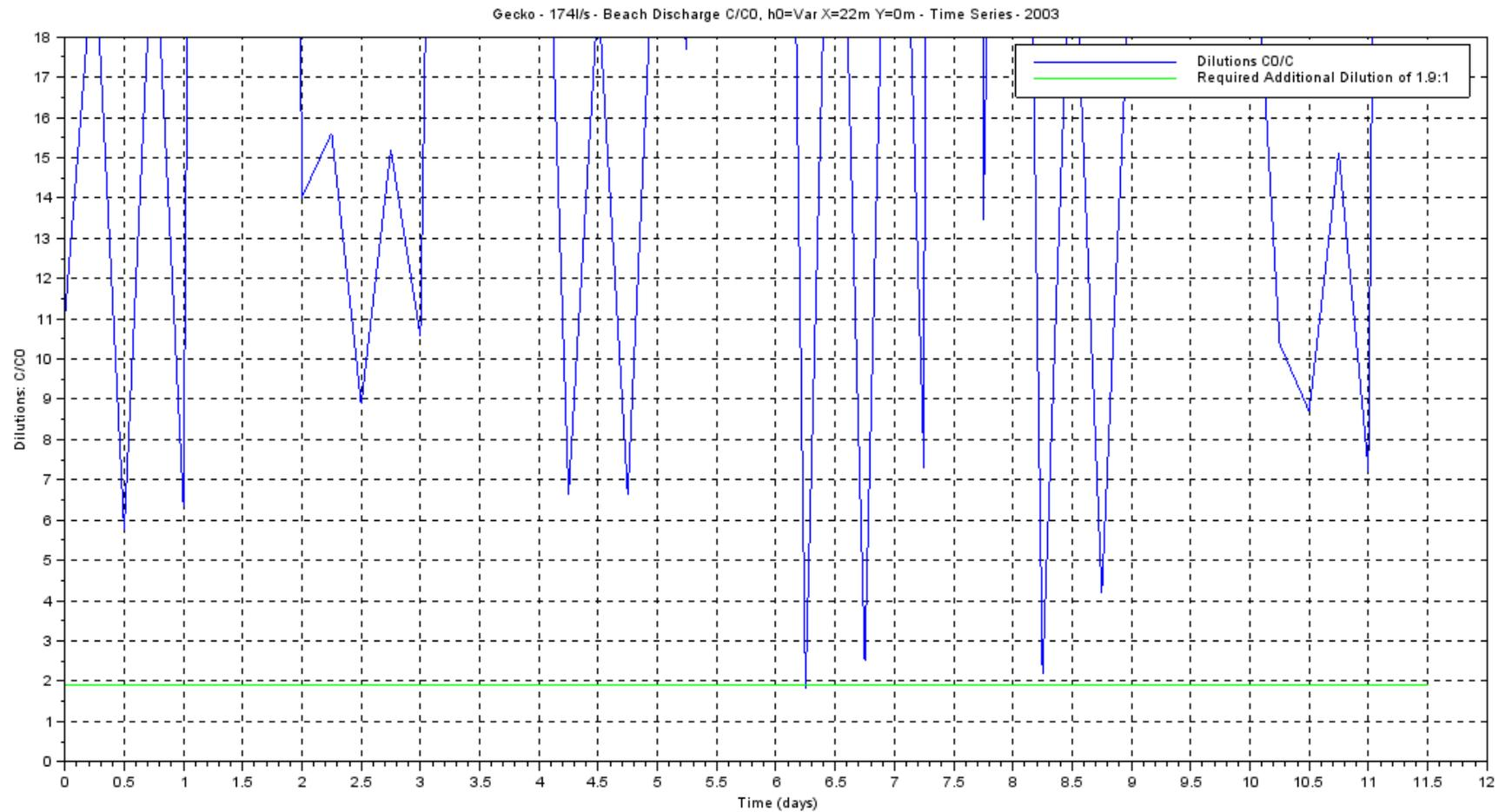
Figure 8.5: Plot of dilutions achieved for the 2003 time series calculated at a fixed point “E” (22m from the point of initial dilution) for the brine effluent discharge. The green line indicates the required dilution of  $D=1.9:1$ . The blue peaks below the line indicate dilutions below the required  $D=1.9:1$ .
