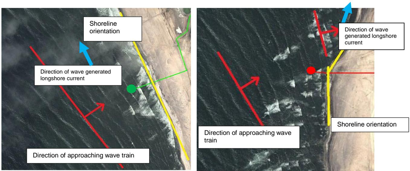
Wave train approaching the proposed southern discharge site. Note the approaching wave train is approximately parallel to the shoreline orientation.
