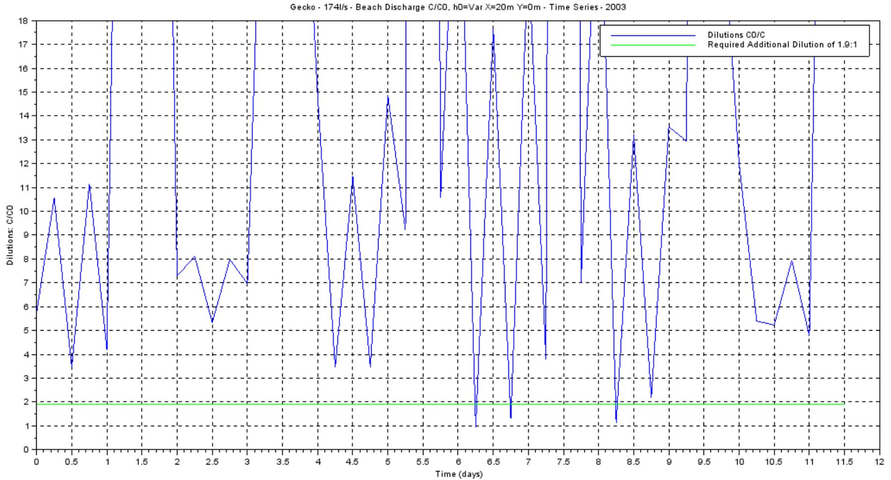
Figure 8.4: Plot of dilutions achieved for the 2003 time series calculated at a fixed point “D” (20m from the point of initial dilution) for the brine effluent discharge. The green line indicates the required dilution of  $D=1.9:1$ . The blue peaks below the line indicate dilutions below the required  $D=1.9:1$ .
