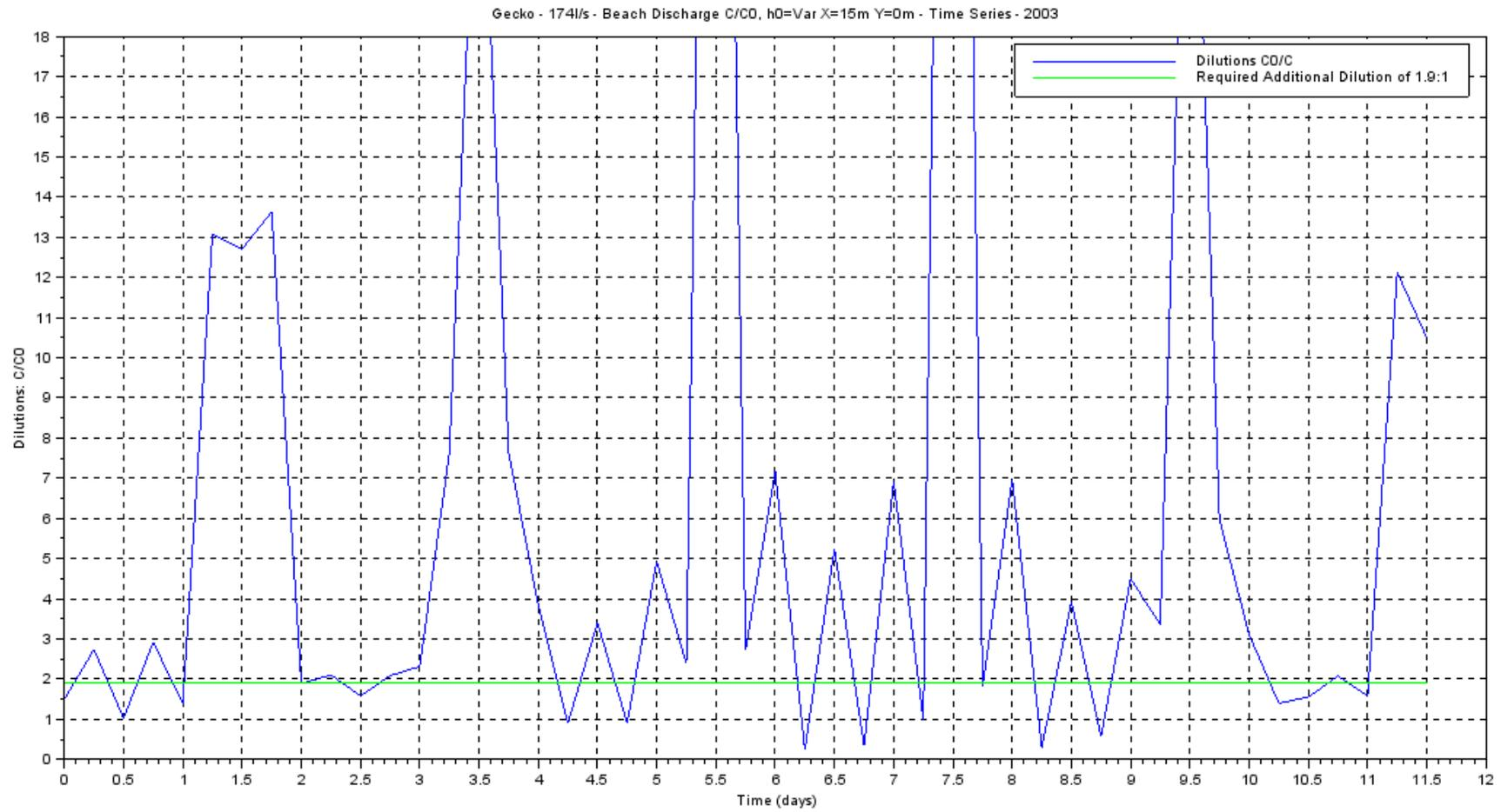
Figure 8.3: Plot of dilutions achieved for the 2003 time series calculated at a fixed point “C” (15m from the point of initial dilution) for the brine effluent discharge. The green line indicates the required dilution of  $D=1.9:1$ . The blue peaks below the line indicate dilutions below the required  $D=1.9:1$ .
