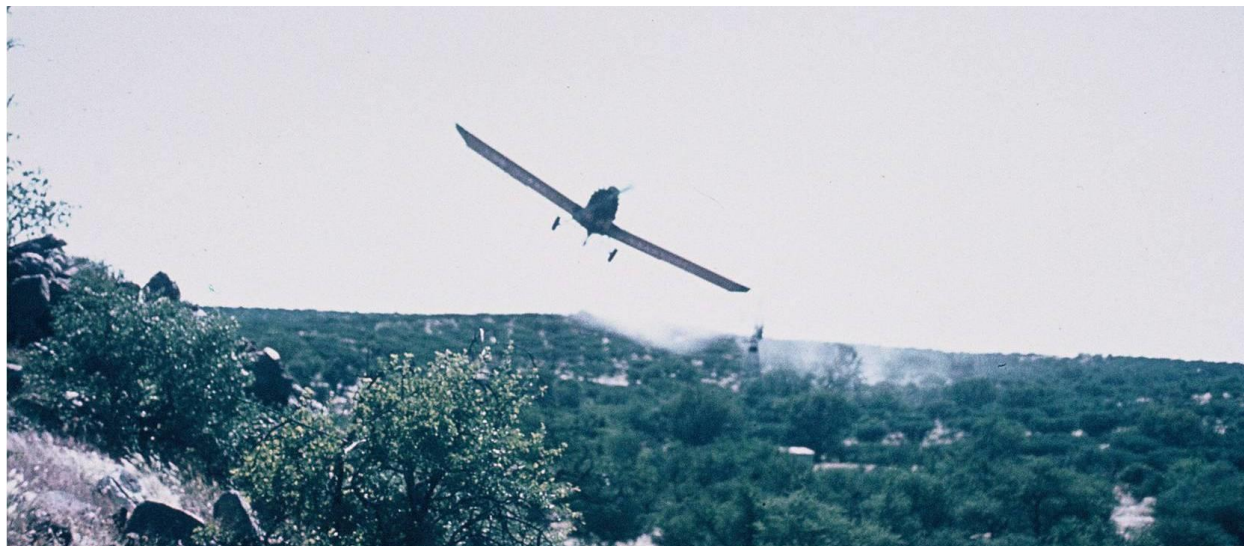
Picture 4: Small planes used to broadcast arboricides from air, for mass bush control
