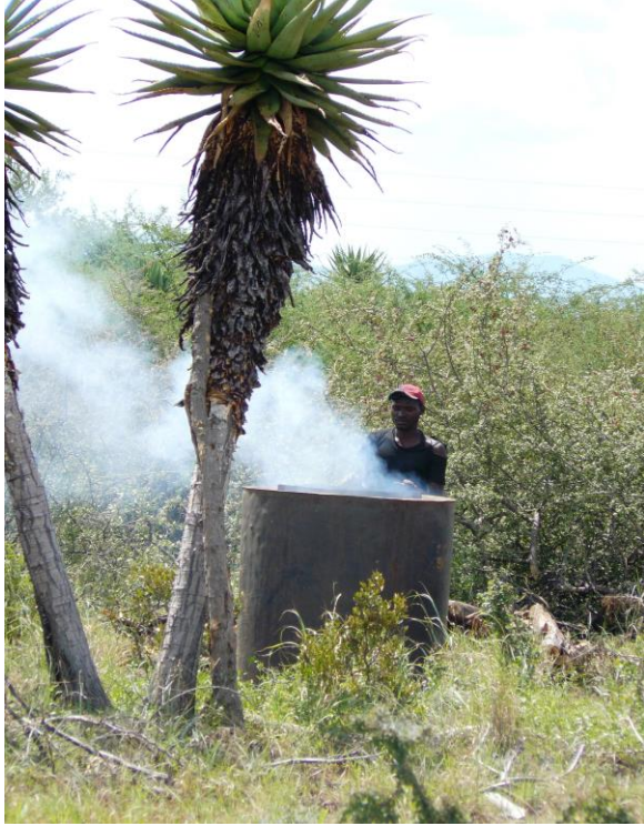
Picture 6: Charcoal from partially burning wood in kilns
