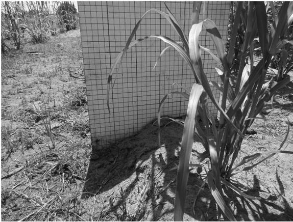
Fig. 3. The plate containing 2 cm- grid lines for measuring the profile of the ridge in MP treatment in pearl millet experiment.
