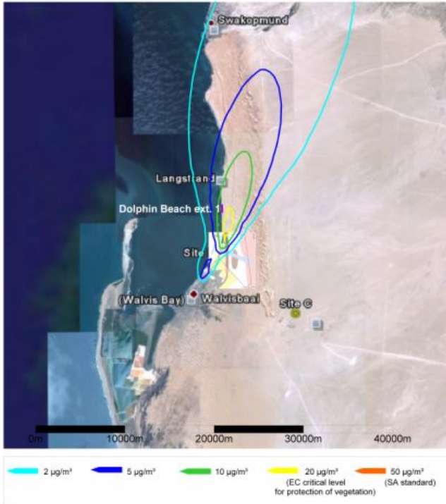
Figure 2. Modelled annual scenarios for SO 2 plumes arising from a power station at Site B South with a 200m high smoke stack, using coal with 1.9% Sulphur content. Fig 2a shows plumes from a 400MW power station, Figure 2b from a 800 MW one.
