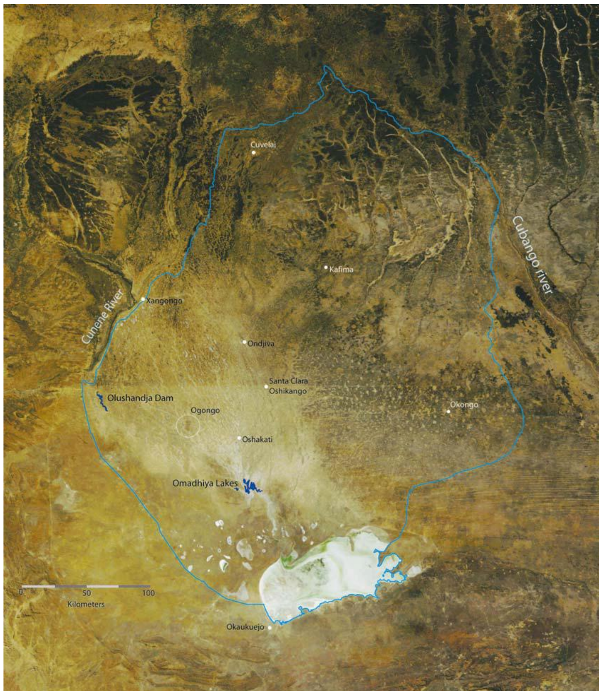
Figure 17: The principal features of the Cuvelai Basin. The pale area south of the border caused by the loss of woodland, and the convergence of iishana into the Omdhiya Lakes and then into Etosha Pan. Olushandja Dam was built to store water from the Cunene River (Source: Mendelsohn, 2011).
