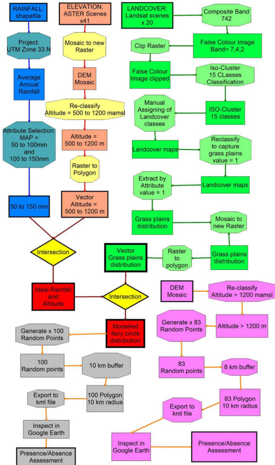
Figure 3.9: GIS model. Blue corresponds to determining the ideal rainfall range, the orange part corresponds to determining the ideal altitude range and the green part determining the ideal land cover. The grey area represents the validation part of the modelled fairy circle distribution, while the purple area represents the control.
