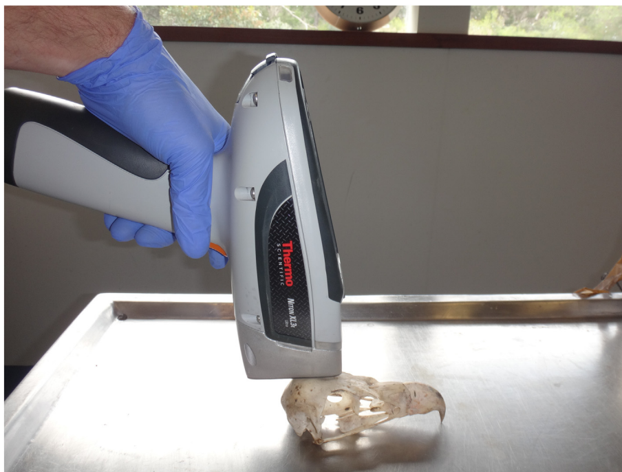
Fig. 1. Methods used to measure bone lead concentrations via X-ray fluorescence (XRF) in bare skulls of wedge-tailed eagles ( Aquila audax audax ) from mainland Australia.
