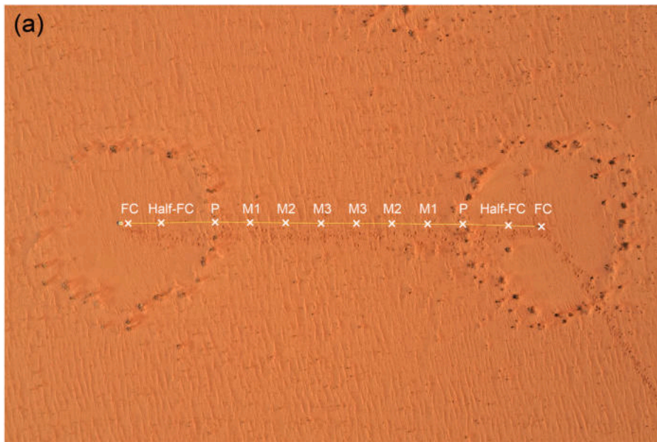
Fig. 5. Continuous soil-moisture measurements from dry to rainy seasons at Jagkop. Drone image of the two FCs without grass cover, taken on 18th February 2020 (a). The right “FC-1” is 7.0 m in diameter and the left “FC-2” measures 7.7 m. Soil-moisture sensors were placed at 20 cm depth and regular distances along the measuring tape. The distance between the two FC centers is 19 m. Results for soil-moisture recordings around “FC-2” (b). Two main rain events occurred in 2022: one on 21st January and one on 14th February. Two minor rain events occurred in between. Data were recorded until the 1st of April 2022. Without matrix grasses after initial rainfall, the drop in soil-water was very slow at all sensor positions (left blue line). But with a dense cover of transpiring grasses in the matrix a month later, the water loss in the unvegetated FC and in the matrix was very fast (right blue line). The data logger with “FC-2” is shown together with the dry matrix grasses on 1st April 2022 (c).
