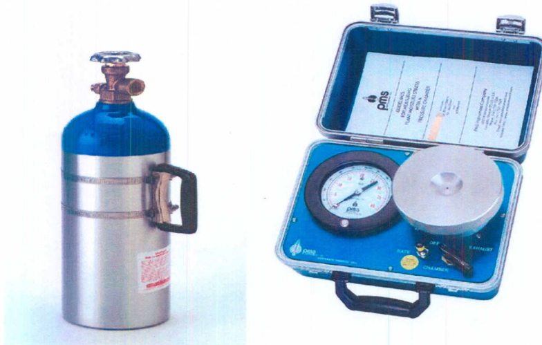
Figure 1: Pressure tank, PMS instrument with pressure chamber
