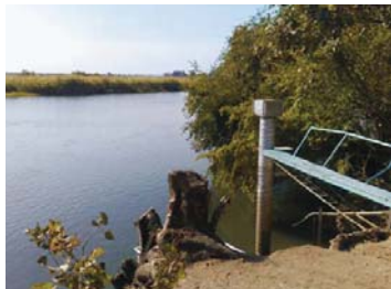
The gauging station at Mohembo where Botswana measures the volume of water entering the Delta.
