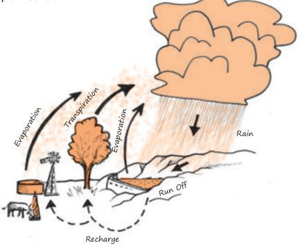
This is a simplified diagram of the water cycle. Rainwater runs off and either infiltrates the soil. runs into the rivers. or fills dams. It refreshes the *aroundwater and allows* plants to grow. Rainfall is the main element that makes our land productive - without rain no plants can grow, animals die of hunger and water sources remain dry. However, the high evaporation rate means that much of the rain returns to the atmosphere.
