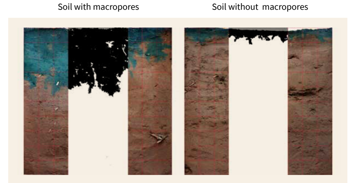
Figure 1: Example of an adjusted 50 x 50 cm infiltration profile picture on loamy soil with macropores (left) and its control plot without macropores (right). The blue colour showing the infiltration depth in the sandy soil profile is a common food colourant. The black and white parts show the inner 20 cm of the pictures used for the analysis.
