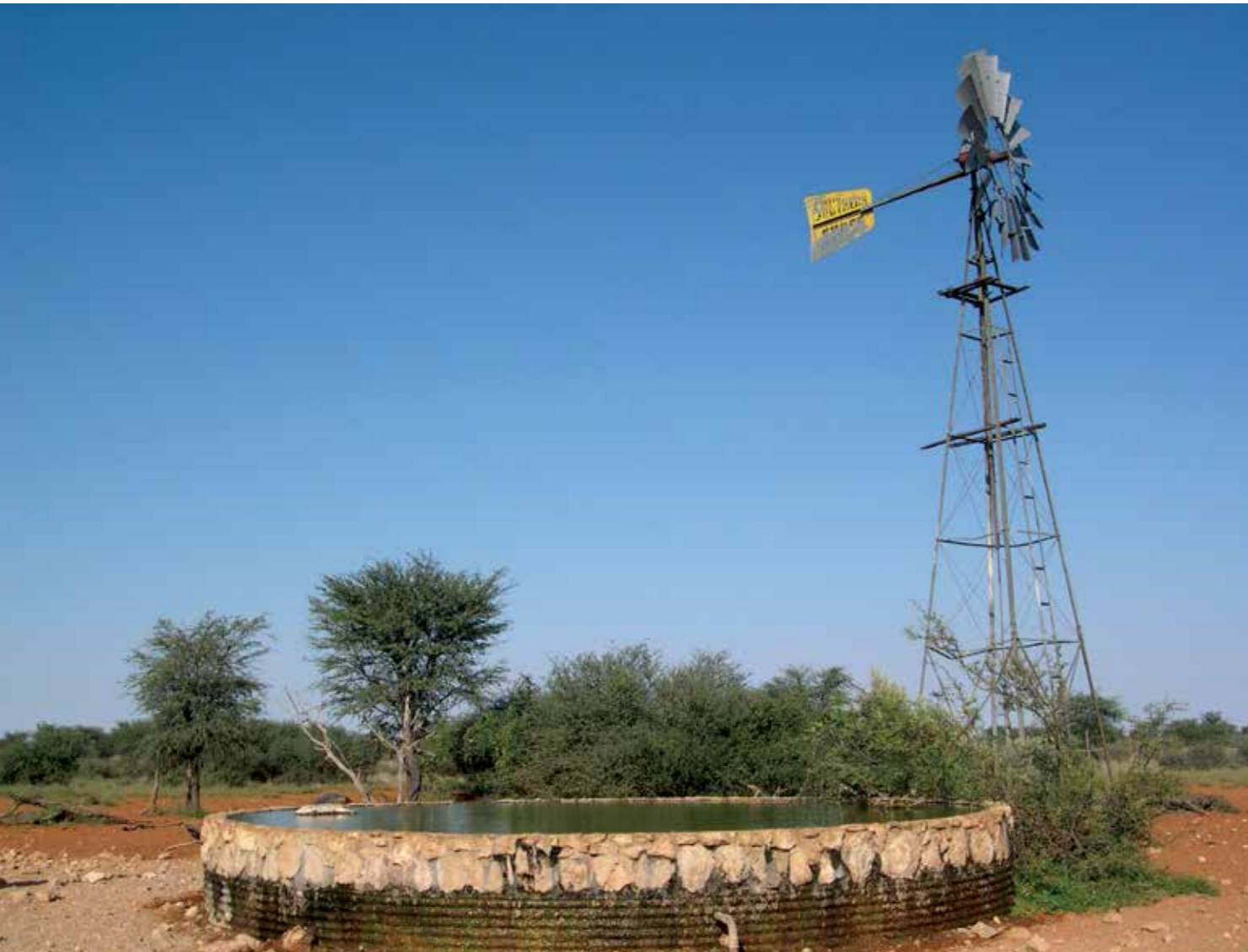
Water basin with a wind-driven pump for drinking animals on a cattle farm in East Namibia
