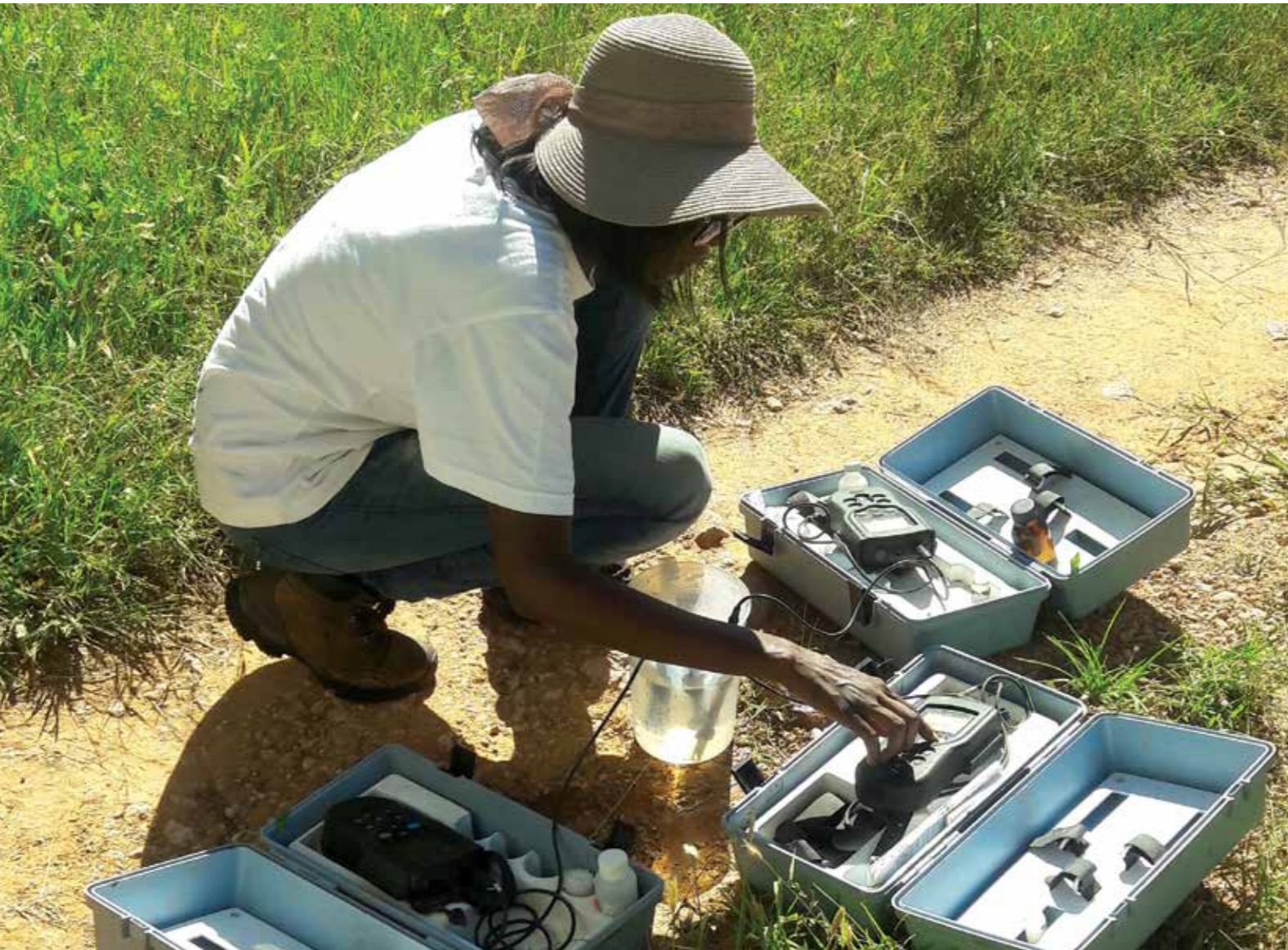
Shoopala Uugulu measuring of groundwater parameters in the field
