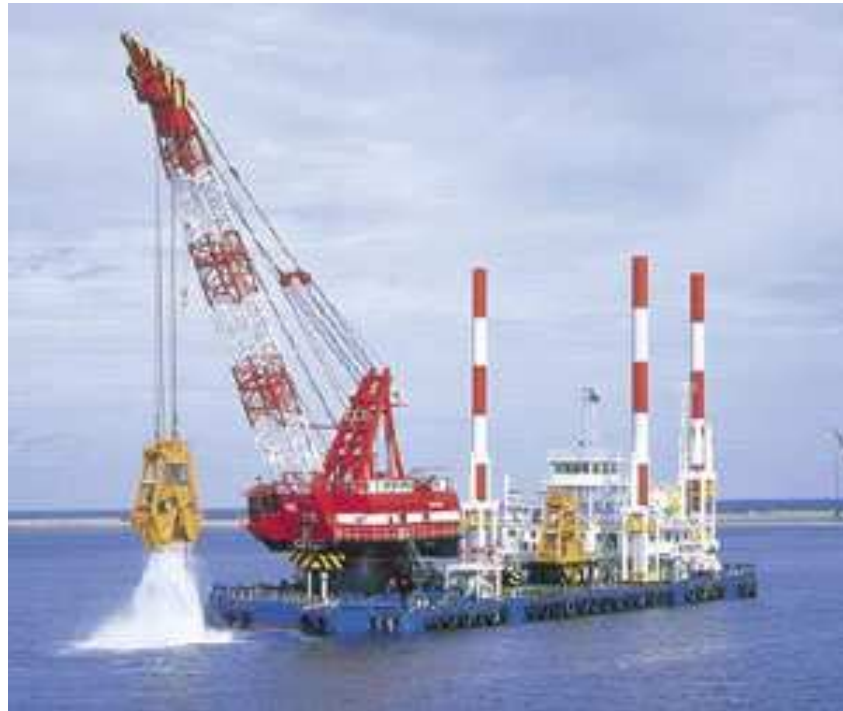
Figure 3.10 Example of a grab bucket dredger
