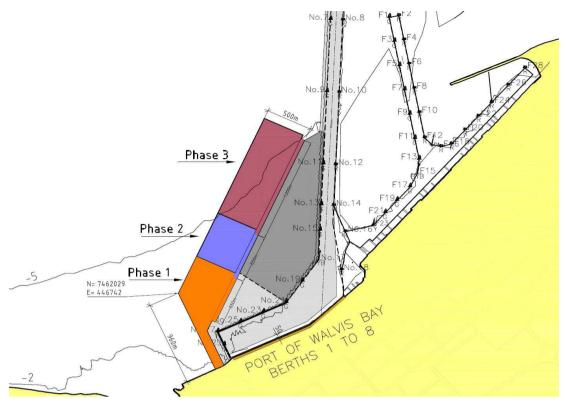
Figure 1: Three phases of proposed container terminal expansion
