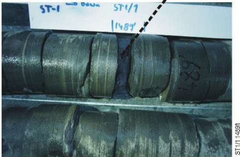
Figure 29: Core sample from the ST-1 well, depicting black shales at 1,489-foot depth
