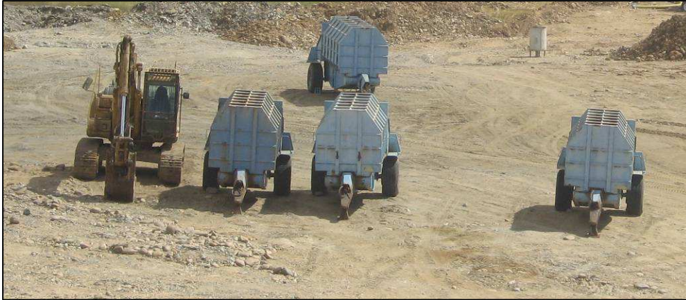
Figure 3.7 Typical transvac suction units used at Orange River Mines.
