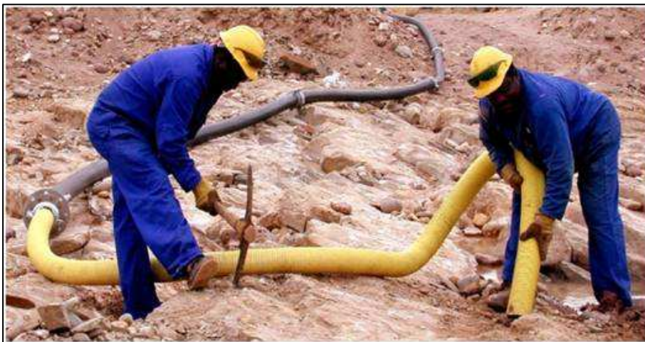
Figure 3.8 The footwall (bedrock) in some zones will be thoroughly cleaned using industrial vacuum units to ensure the recovery of all diamonds.
