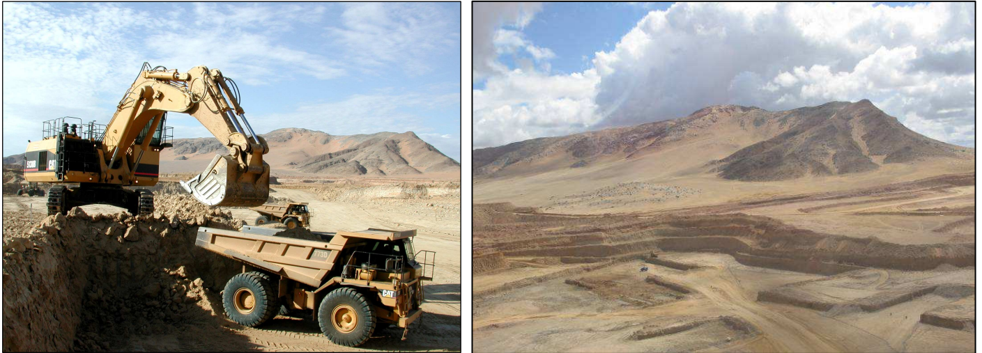
Figure 3.4 Sendelingsdrif will be exploited with conventional open pit mining methods.
