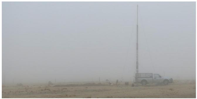
"Gobabeb-Met", one of nine similar weather stations that make up the FogNet array, being constructed in thick early-morning fog at the Centre. The other eight stations are arranged in two transects, one (E-W) from the coast to about 80km inland, and one (N-S) along the 400-500m altitude contour. As main reference station, Gobabeb-Met received more instruments than the others.
