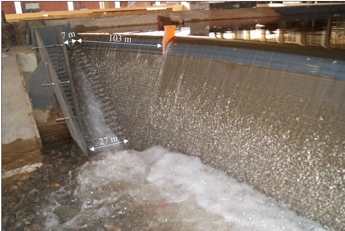
Fig. 5. Option 4: Flow depth on the spillway chute where the last 103 m of the Ogee crest was raised by 2.4 m and the dimensions of the chute was 7.0 m on the top and 27 m at the bottom during the RDD
