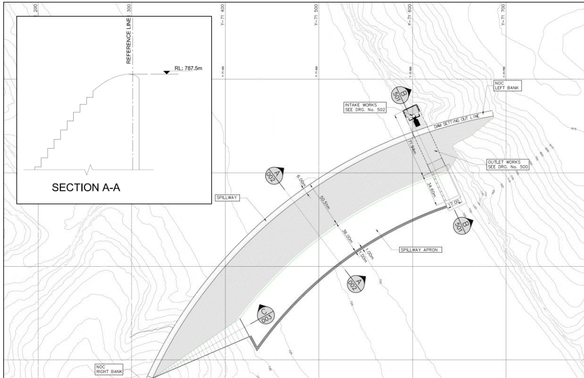
Fig. 1. Plan of the preliminary design of the Neckartal Dam (Top left insert: uniform Ogee spillway section)
