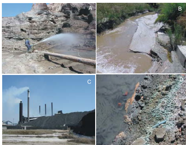
Figure 6. Source of the contamination of the Kafue River sediments. A: Washing out (re-working) of old flotation tailings for chemical leaching, Chingola area. Due to an insufficient volume of the retention reservoir, suspension of tailings overflow the retention dam. B: Siltation of the Changa River (Chambishi Area) with outflow from waste heaps. C: Slag deposits at the Nkana (Kitwe) Smelter. D: Washout from slag deposit is one of the important sources of contamination of the Kafue River sediments.
