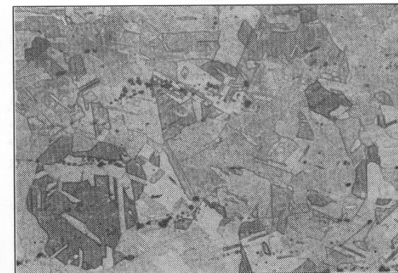
Figure 9: Etched section of bead KIN 1 showing recrystallised copper grains with annealing twins (124 X)
