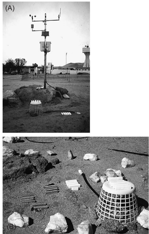
Fig. 3. Experimental setup at Gobabeb: (A) automatic meteorological station with rock surface temperature probe and exposure blocks in front; and (B) detailed view of rock surface probe, weathering platform, and granite and marble exposure blocks.
