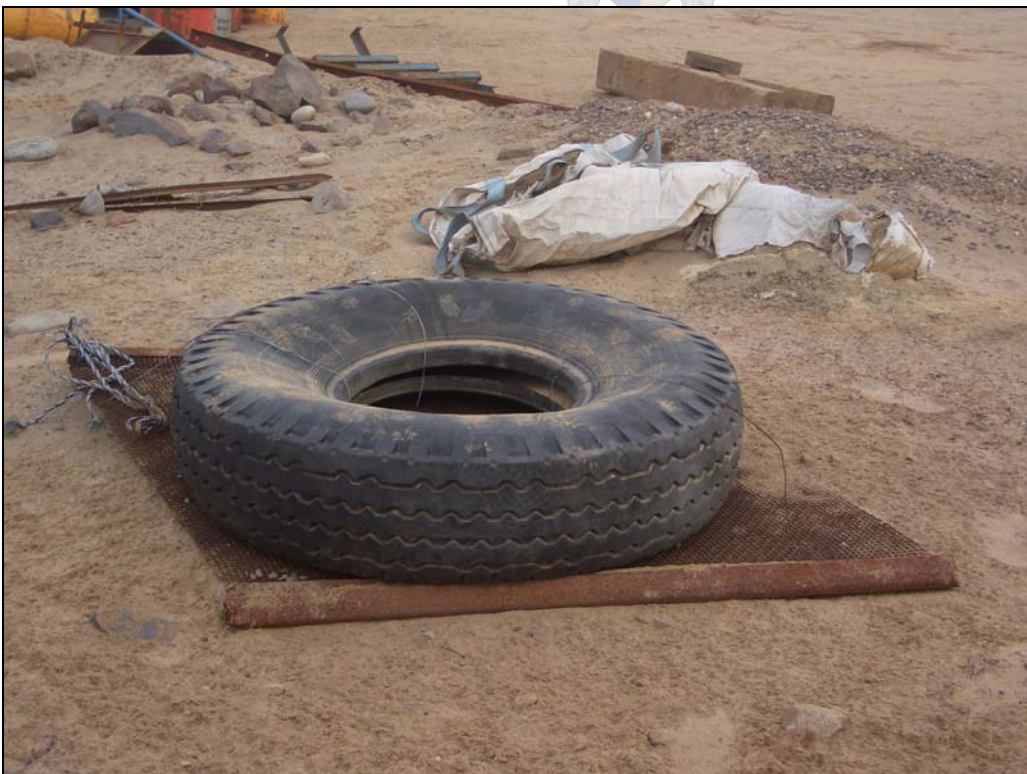
Figure 5.9 'Tyre and grid' contraption for smoothing disturbed surfaces
