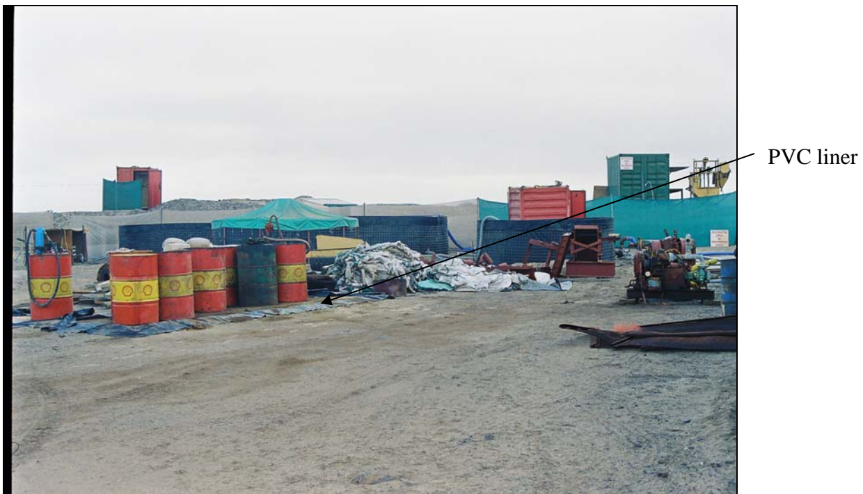
Figure 5.2 Oil drums stored on a PVC liner
