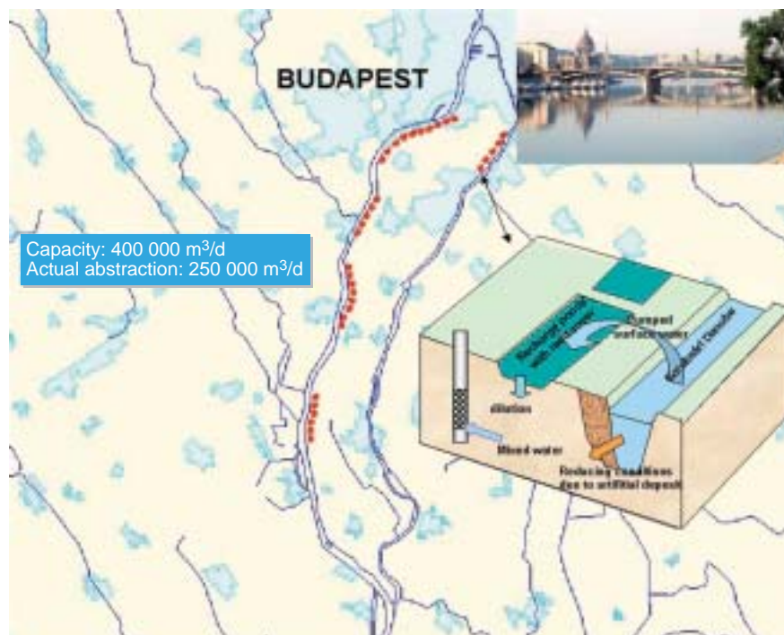
Figure 9. Qualitative improvement of bank filtered water with artificial recharge at Szigetszentmiklós.
