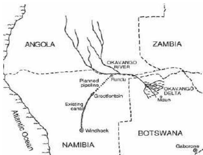
Map 3: “The Rundu-Grootfontein Pipeline”. The graphic shows the location of the proposed Namibian pipeline (Source: Ramberg 1997).
