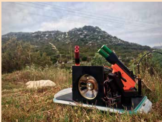
Figure 6.3. Virtual fence, Mark I-model, remote controlled action station. Note the two double-barrelled bearbanger guns, loaded with banger (red) and whistler (green) flares, and one high ampere speaker. The Mark III-model action stations are fully waterproof and have two speakers and only one gun. Photo: Phillip Richardson.
