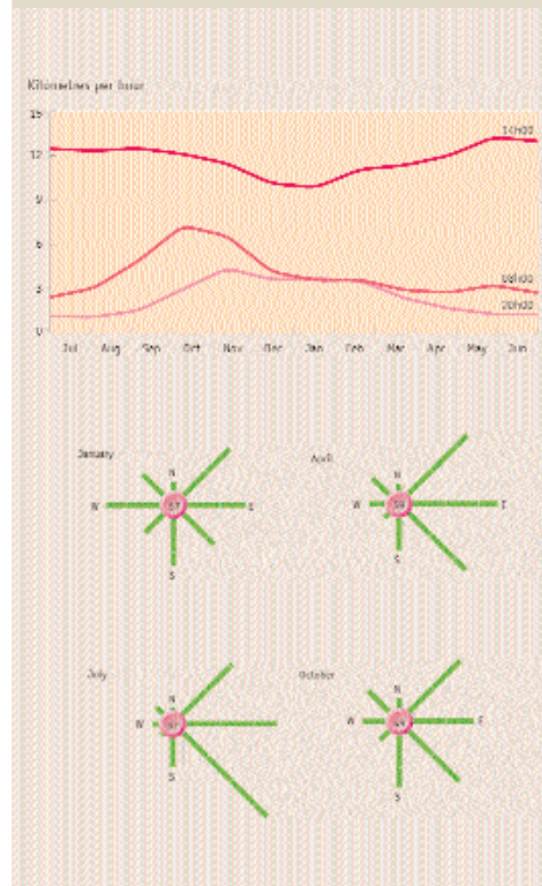
FIGURE 19- Kavango is not a windy place, and it is calm for over half the time. The graph shows average wind speeds measured in Rundu at eight in the morning, two in the afternoon and at eight in the evening. Wind roses show the proportions of time recorded from different directions in January, April, July and October. The numbers at the centres of each rose are the percentages of time that it is calm.
