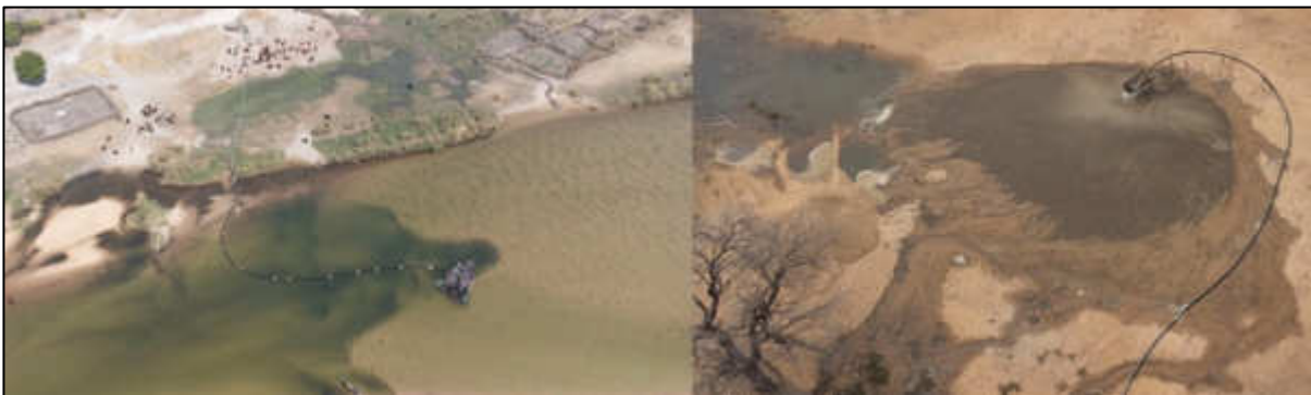
Figure 15: Dredgers were used to mine building sand from the Kavango river (left) or to sift it for unknown reasons (right).
