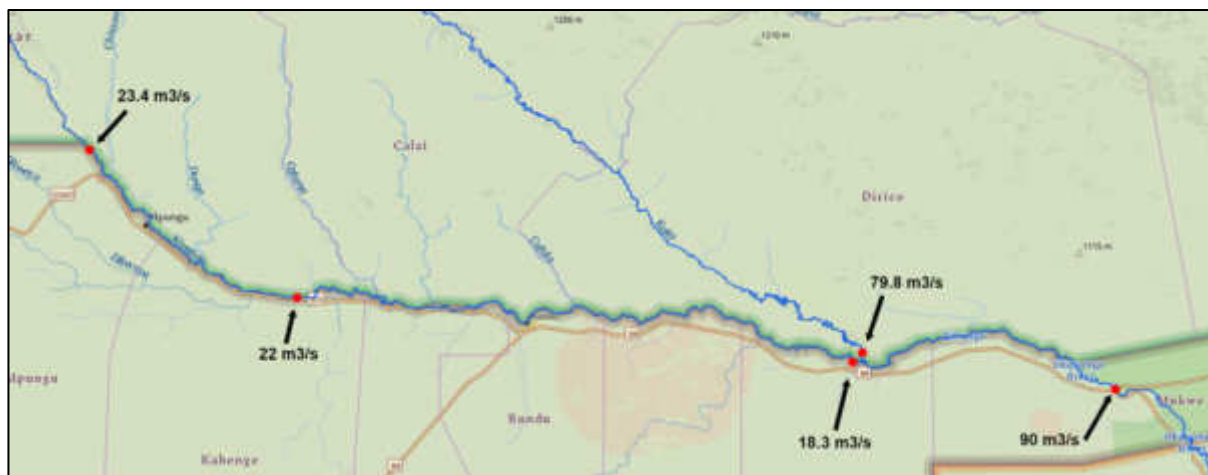
Figure 33: Discharge rates along the Kavango River calculated using ADCP between 30 August (Katwitwi) and 17 September (confluence), 2021.
