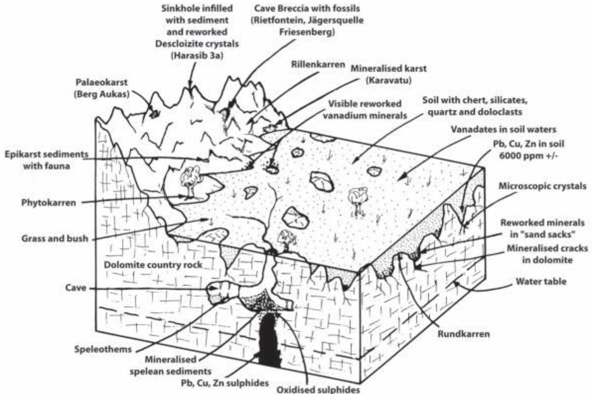
**Figure 20.-** Reconstructed geomorphology of a karst terrain in the Otavi Mountains showing some of the main features including locations of massive sulphides, vanadium mineralisation and fossiliferous karst infillings. There is a clear karstic control on the localisation of vanadium deposits and fossil sites.
