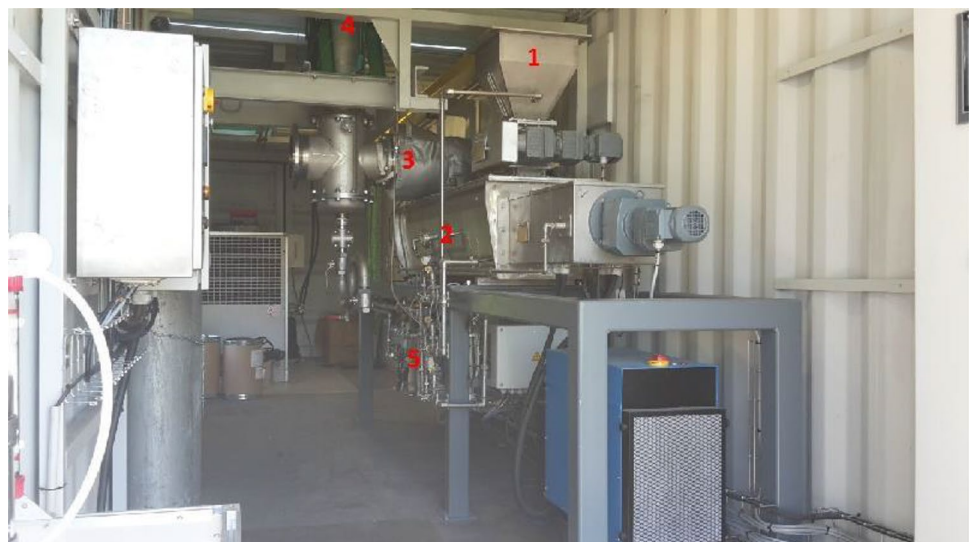
Fig. 2 The pyrolysis chamber. Source: Author’s Compilation (2017)
