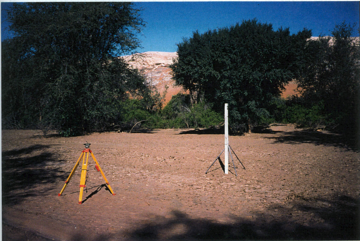
Photograph 3.3b Dumpy level and staff used for the survey
