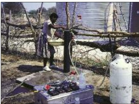
Isotope sampling of a solar powered well in the Northern Central area
