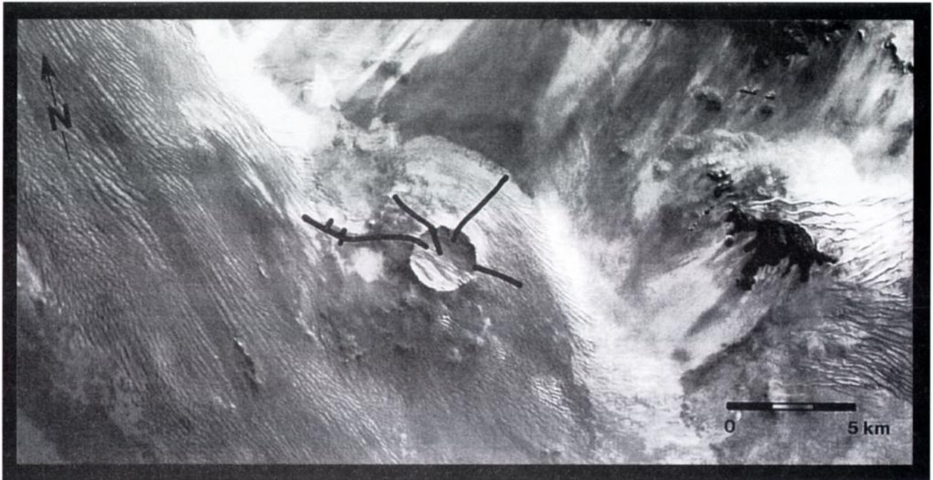
Figure 1. Landsat thematic mapper (TM) view of the Roter Kamm impact crater and vicinity, Namibia (centered at 27°46'S; 16°18'E). Black lines mark the location of GPR transects completed in and around the crater. Transects shown are longer than 100 m: numerous shorter transects were completed within and outside of the crater but are not displayed. Image resolution is 30 m/pixel.
