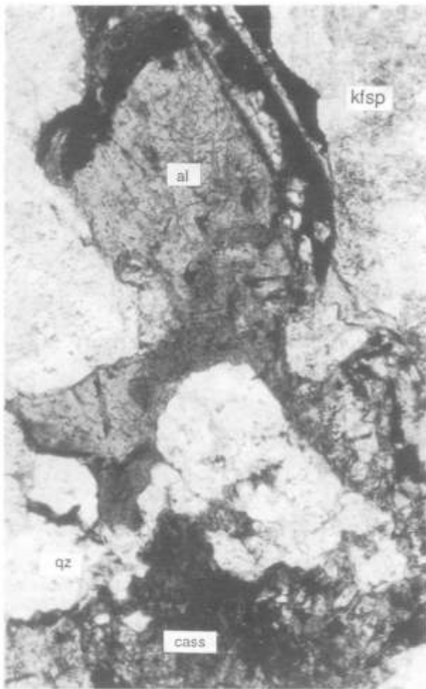
Fig. 63: Photomicrograph of zoned allanite (al), cassiterite (cass), quartz (qz) and alkali feldspar (kfsp) in potash altered biotite granite, Wasserfallfläche (magnification x 41, XPL).
