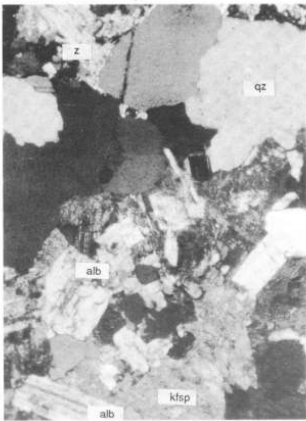
Fig. 19: Photomicrograph of albite-rich biotite granite from the central ring-dyke (magnification x 41, XPL). Quartz (qz), alkali feldspar (kfsp) partly replaced by albite (alb) and colourless, zinnwalditic mica (z).
