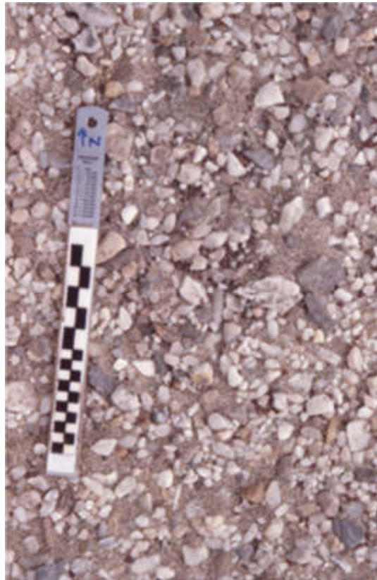
Figure 69. Garnet tracers migrating across a dynamic bedload pavement. Note the presence of discrete grain concentrations which suggest the existence of pathways and preferred sites for segregation of heavy mineral particles. Scale 10 cm
