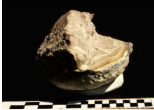
Figure 93. Calcrete pebble with a sub-horizontal step cut into the south face. Had this process continued, the entire clast would have eventually been planed at the bed elevation. Note the small knobs and bosses near the top of the windward face, which formed in response to differential corrosion due to the presence of small quartz grains in the calcrete. Scale 10 cm.
