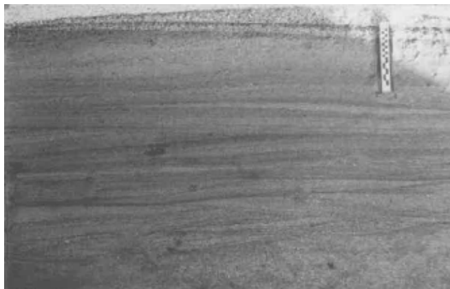
Figure 45. Transverse section through granule ripples showing low-angle stratification. Despite the concentration of granules on the bed there are very few granules in the section which is predominantly sandy. Southerly wind flow out of page. Scale 10 cm.
