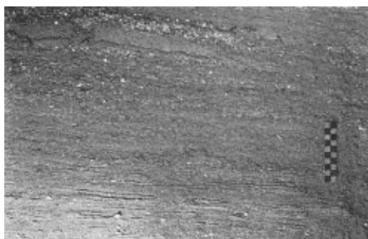
Figure 41. Transverse section through the granule ripple in Fig. 39. Note the low-angle stratification, and concentrations of white granules along bedding planes. Scale in cm.
