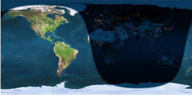
Fig. 2: Binary day-light model for a particular time t . The shape of the dark area depends on the time of the year, and the horizontal position of the dark area depends on the time of the day.
