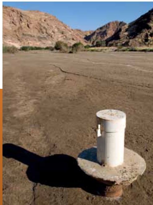
Numbered boreholes have been drilled and equipped for monitoring throughout the project area.
