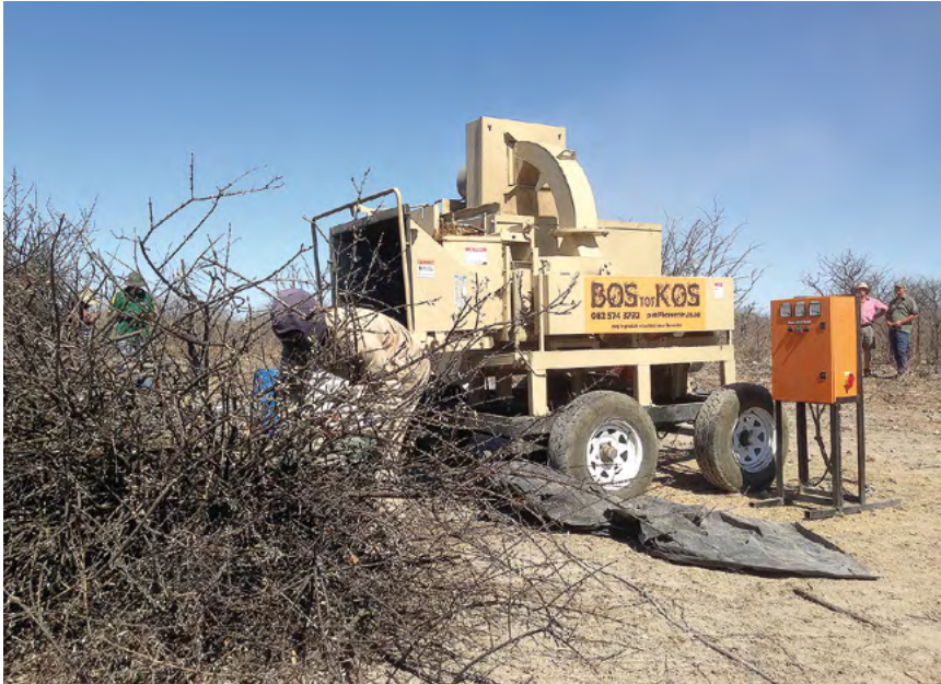
Bush based animal feed production in Namibia, using a combined chipper and feed mixer.
