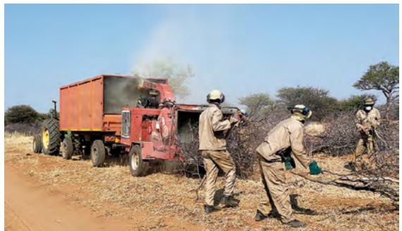
Manual bush harvesting and processing using a chipper
