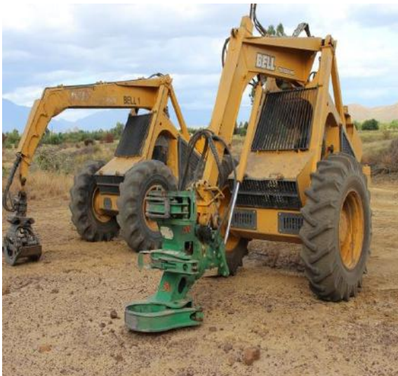
Photograph 6: Three-wheel logger (left) and logger fitted with a hydraulic cutter (right). Courtesy ABC Worcester
