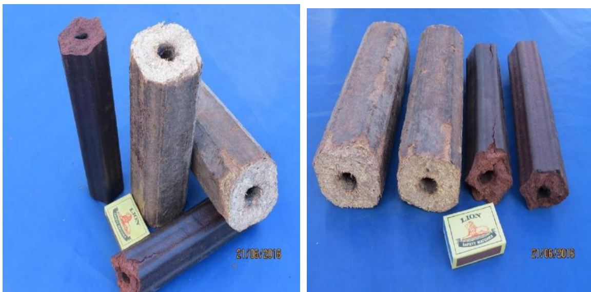
Photographs 25 & 26: Bushblok extrudate and logs from grapeseed
