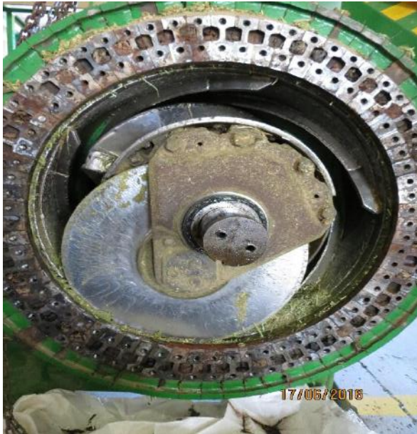
Photograph 29 & 30: A cuber with its front -end wear plate removed
