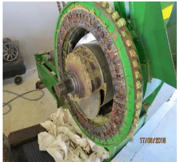
Photographs 13, 14, 15 & 16: A Cuber machine with its front wear plate removed to expose the 66 removable dies and excentric press wheel
