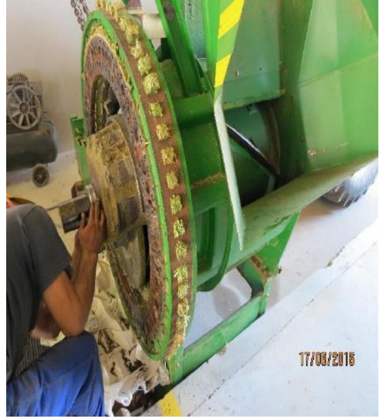
Photograph 29 & 30: A cuber with its front -end wear plate removed
