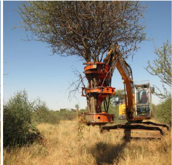
Photograph 4 & 5: Felling of bush using a hydraulic cutter (WoodCo)
