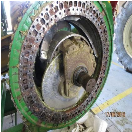
Photographs 13, 14, 15 & 16: A Cuber machine with its front wear plate removed to expose the 66 removable dies and excentric press wheel
