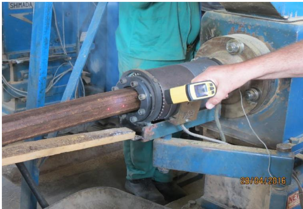
Photograph 19: Measuring the surface temperature of a Bushblok exiting the heated barrel
