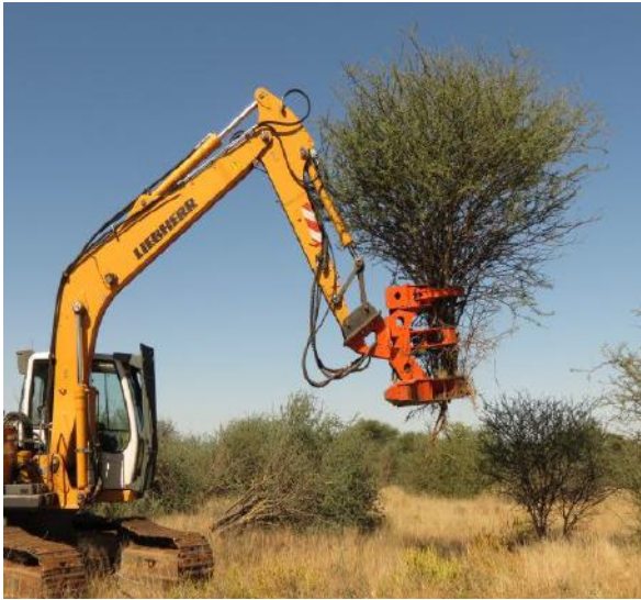
Photograph 4 & 5: Felling of bush using a hydraulic cutter (WoodCo)
