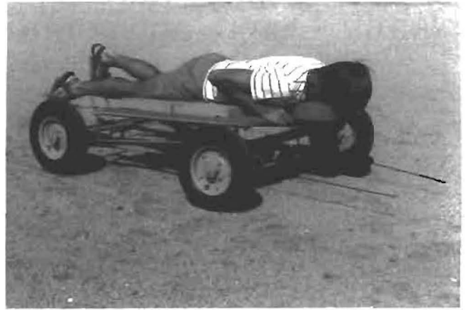
Figure 2 Vehicle used to census foraging ants. Note the two antennae demarcating a 50 cm wide transect.
