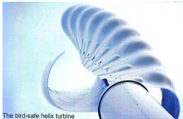
Figure 4 - Close up view of the bird friendly Helix wind turbine
