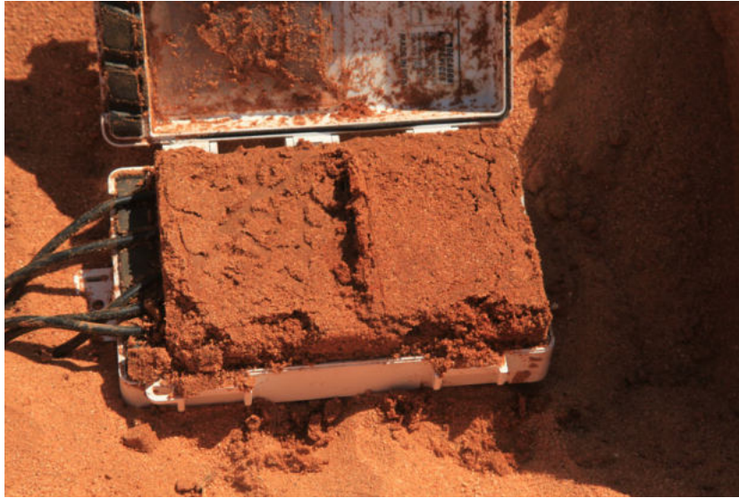
Figure 5. A logger for storage of the soil moisture data located in dry sand at 10 cm below the soil surface is found filled with very moist sand brought in by Psammotermes termites (Giribesvlakte, Namibia, 19 May 2015). (Online version in colour.)
