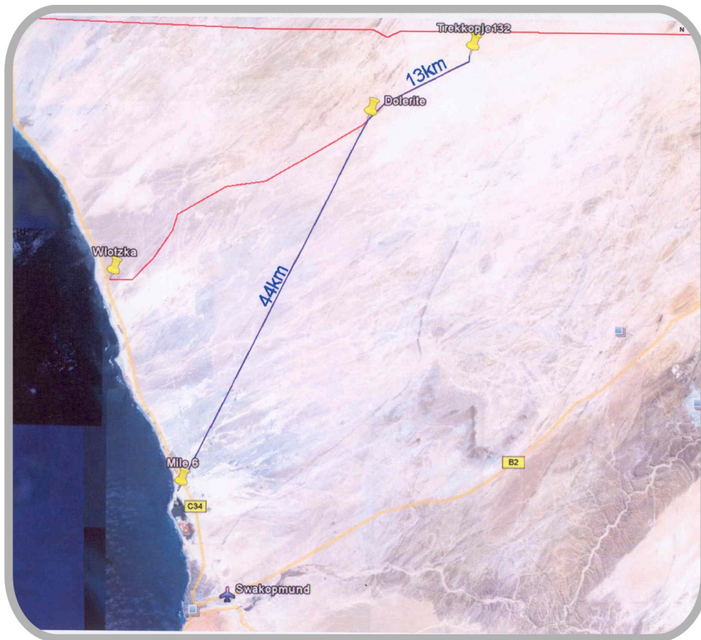
Figure 2.4: Proposed route for a new 132 kV transmission line of 44 km from the existing Dolerite line to the new substation at the Mile 6 site
