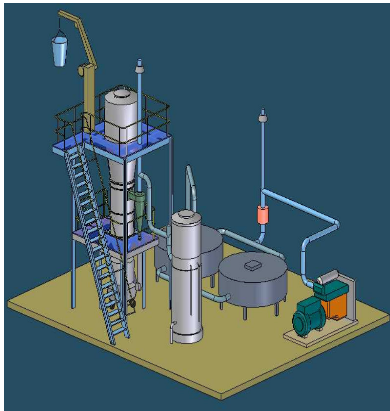
Figure 3: Schematic of a small gasification plant 13
