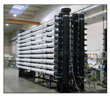
Figure 4 - NORIT Seaguard Ultrafiltration Skid
